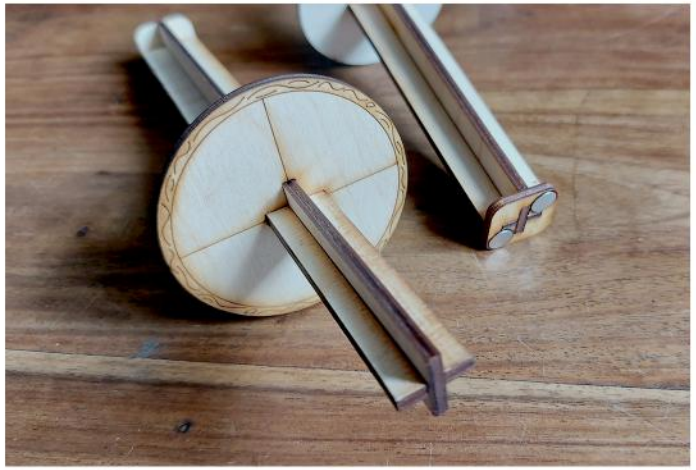
19) Glue and slide the two main sections of the mast together, then glue on the crow's nest panel with the texture facing upwards and finally glue on the base panel ensuring the magnets are facing downwards.
