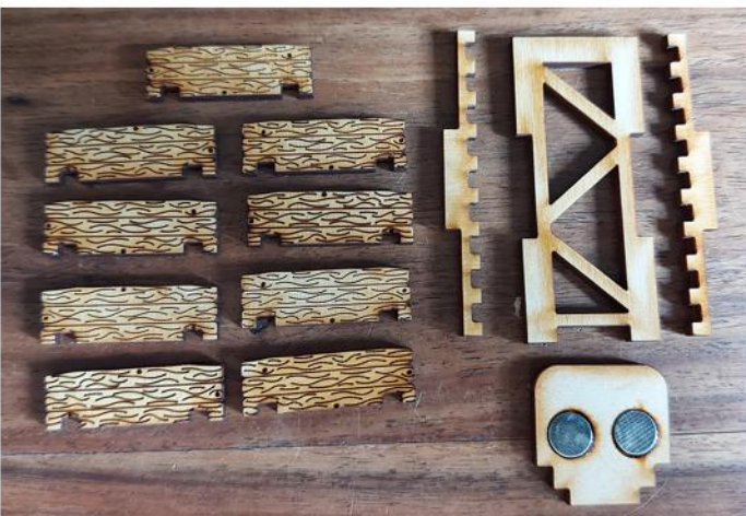
28) Layout of all the parts needed to assemble the lower deck staircase. x1 Back wall panel, x2 Stair side panels, x1 magnetic base panel, x9 stair panels.
