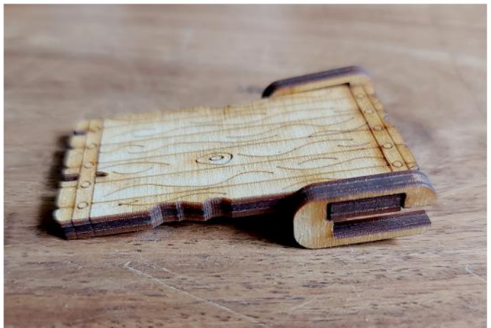
23) Assemble the plank as shown above, apply glue to both side clips, ensure they are facing the right directions (towards the deck) before gluing in place.
