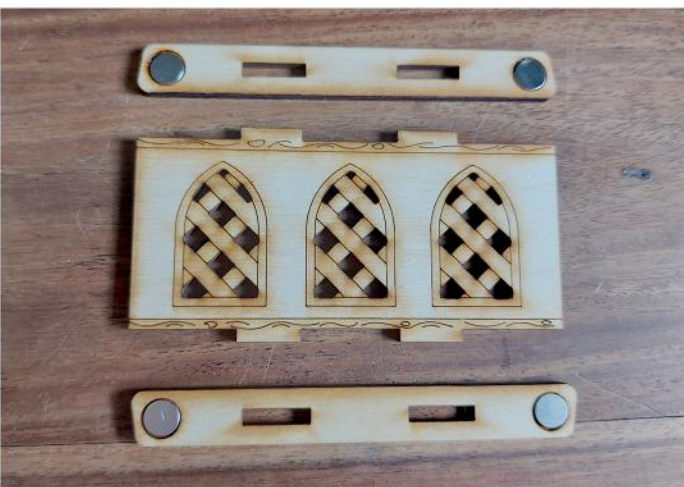
10) Layout of all the parts needed to assemble the window panel. Before gluing the panels into place, make sure you have checked the magnets against the Main deck and Top decks corresponding magnets.
