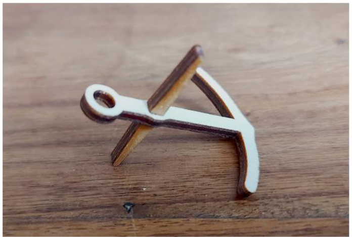
21) apply a small amount of glue to the tabs of both the anchor arms and slide them into the square hole on the main anchor body as shown above.
